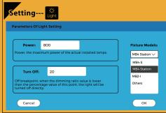
Fixture Models: Choose the correct fixture model for connection. Both wired and wireless connections are suitable for MB4 Station, MB4-S and MB2-I; Others could only be controlled by wired connection.
